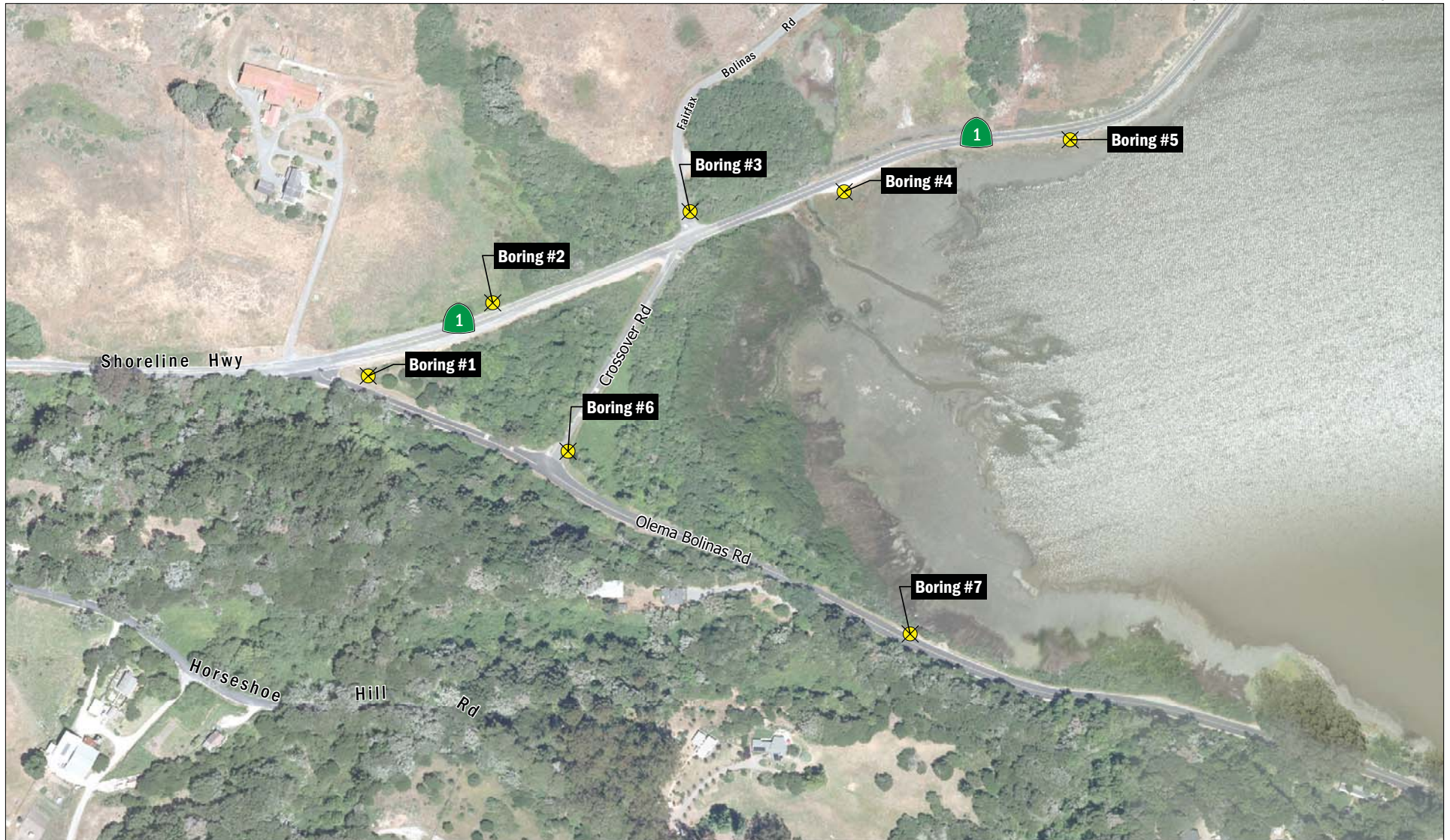
FIGURE 1 Project Site and Geotechnical Boring Location Plan, June 2017
